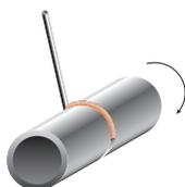
**PA TUBE EN ROTATION.** L'AXE DU TUBE EST HORIZONTAL.
