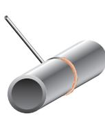
**PF TUBE FIXE.** L'AXE DU TUBE EST HORIZONTAL.
