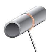
**PG TUBE FIXE.** L'AXE DU TUBE EST HORIZONTAL.
