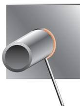
PG TUBE FIXE. L'AXE DU TUBE EST HORIZONTAL.
