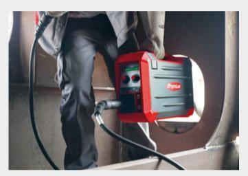
/ An ergonomically designed carrying handle makes for safe transport and handling – manually or crane-lifted by cable.
