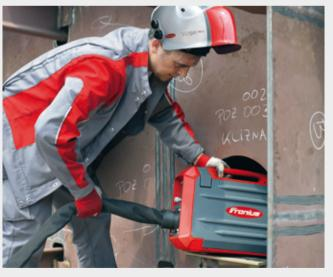
/ Weighing less than 10 kg (22.05 lb) and with minimal obstacle contours, the VR 5000 Case fits through any manhole commonly found in shipbuilding, down to 350 mm (13.8 inches).
